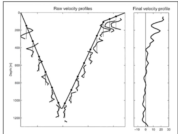
ADCP profiles are stitched together to form a full-depth profile. Speed (cm/s).
